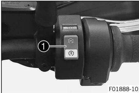
The emergency OFF switch/electric starter button ❶ is located on the right side of the combination switch.
