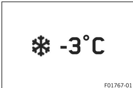
The ice warning ❄ goes on when there is an increased risk of ice on the roads. The ice warning ❄ appears on the display when the ambient temperature drops below the specified value.
